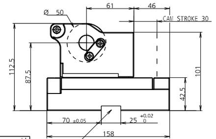
We suggest you to assembly by using a thrust mount key
