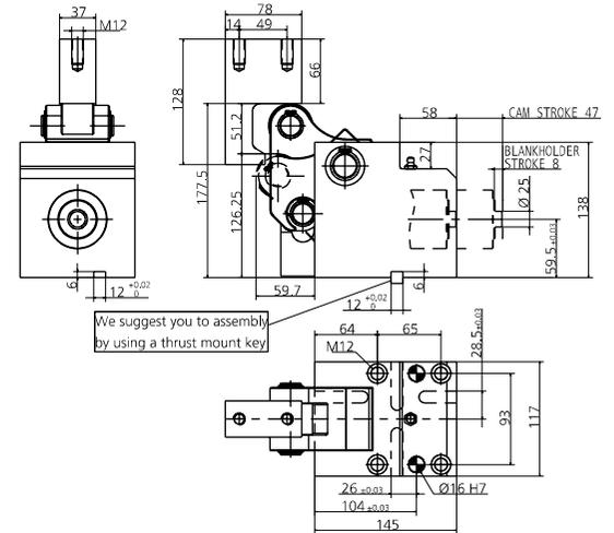
We suggest you to assembly by using a thrust mount key
