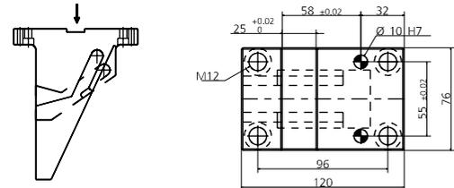
019 (9003) SENSORE / SENSOR / SENSOR
