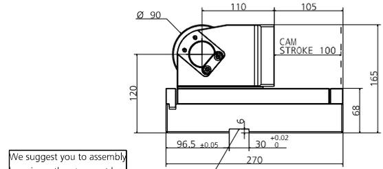
We suggest you to assembly by using a thrust mount key
