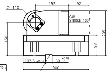
We suggest you to assembly by using a thrust mount key
