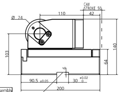
We suggest you to assembly by using a thrust mount key
