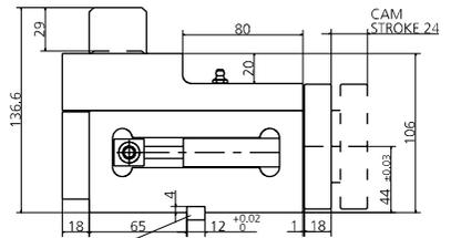
We suggest you to assembly by using a thrust mount key
