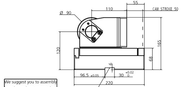
We suggest you to assembly by using a thrust mount key
