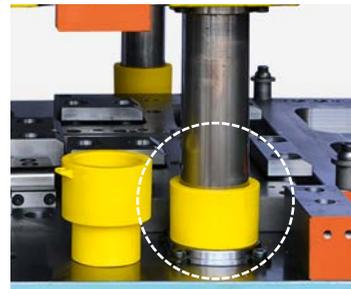
APPOGGIO CASUALE SULLE COLONNE DELLO STAMPO / CASUAL SUPPORT ON THE COLUMNS OF THE DIE / ZUFÄLLIGE UNTERSTÜTZUNG AUF DEN SÄULEN DER MATRIZE / SUPPORT ALÉATOIRE SUR LES COLONNES DE L'OUTIL DE DÉCOUPE
