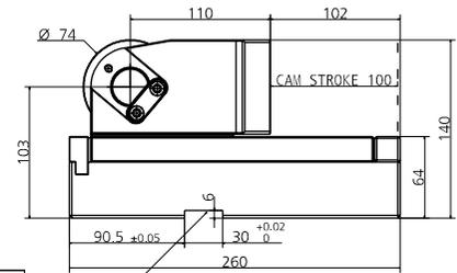
We suggest you to assembly by using a thrust mount key
