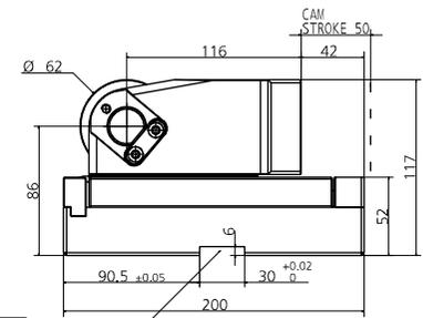
We suggest you to assembly by using a thrust mount key
