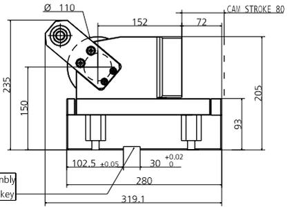
We suggest you to assembly by using a thrust mount key
