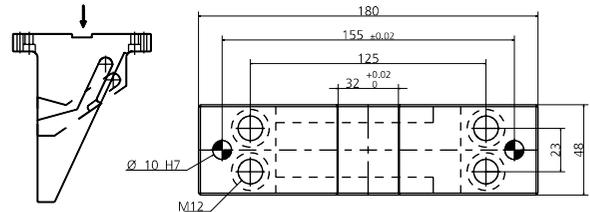
019 (9003) SENSORE / SENSOR / SENSOR
