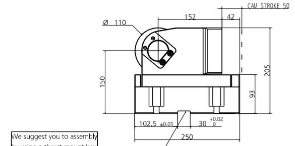
We suggest you to assembly by using a thrust mount key
